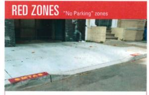
Red zones may be installed near intersection corners, at bus stops, at fire hydrants, at curb ramps or at the edges of driveways.
